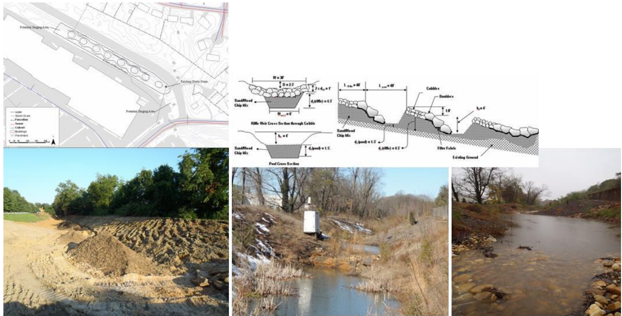
Figure 13. Plan View (top left) and profile and cross section (top right) of the Regenerative Storm Conveyance System; photos (bottom row) showing the system during implementation (left), during normal conditions (middle) and during a storm event (right).
