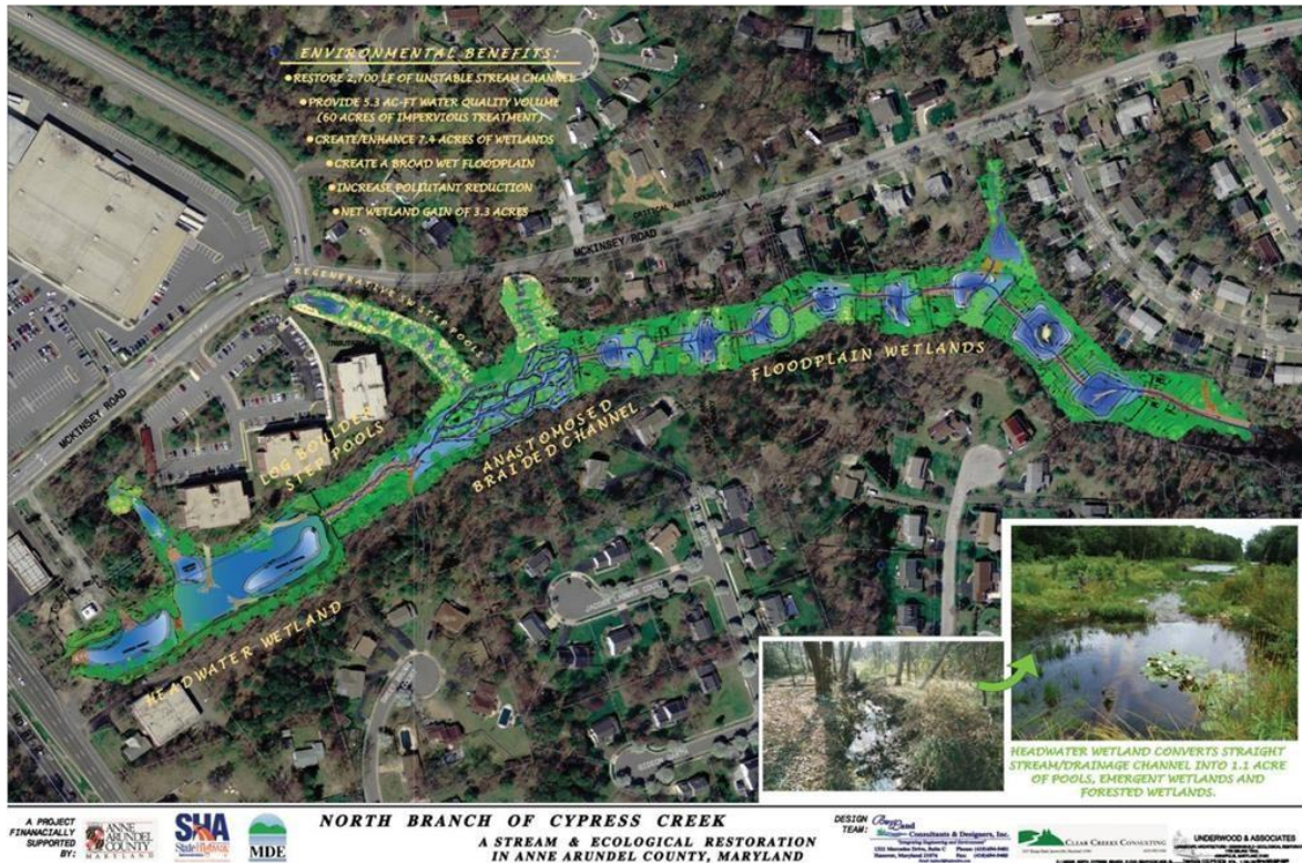
Figure 4. Restoration plans for the North Branch of Cypress Creek, Anne Arundel County, MD, showing a headwater wetland, step pools, an anastomosed braided channel, and floodplain wetlands.
