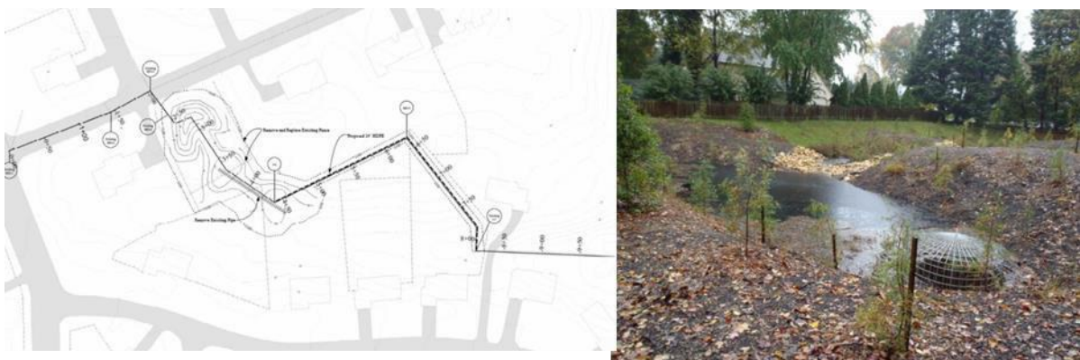
Figure 15. Plan View of the retrofit structure (left) and photo of the Regenerative Storm Conveyance system after implementation (right).
