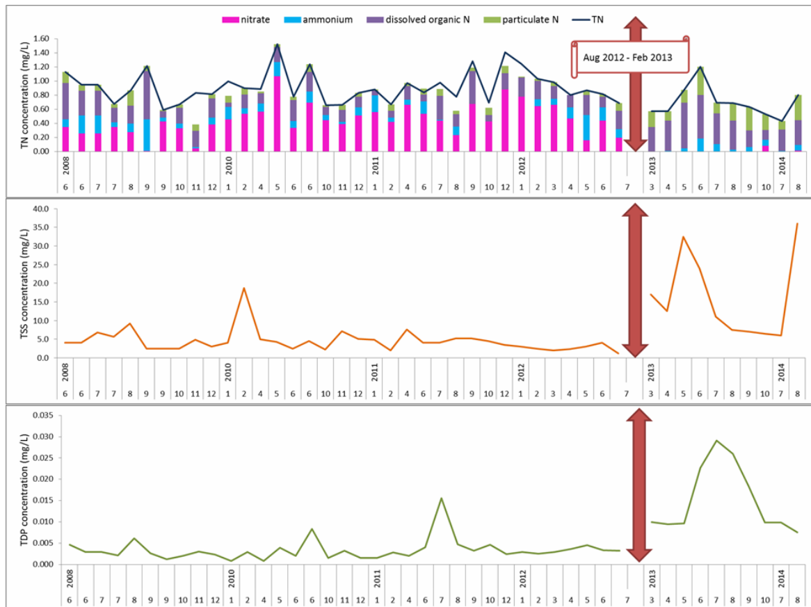
Figure 22a – c (top to bottom). Time series of TN, TDP and TSS concentrations in the baseflow of the north branch of Cypress Creek. Total N is partitioned in different forms (NO 3 , NH 4 , dissolved organic and particulate), pre- and post-construction. Pre-construction concentrations include samples collected since 2008. The construction period (July 2012 to March 2013) is indicated by the vertical red arrow.
